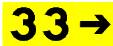
Exhibit 17-Typical Outbound Runway Destination Sign
